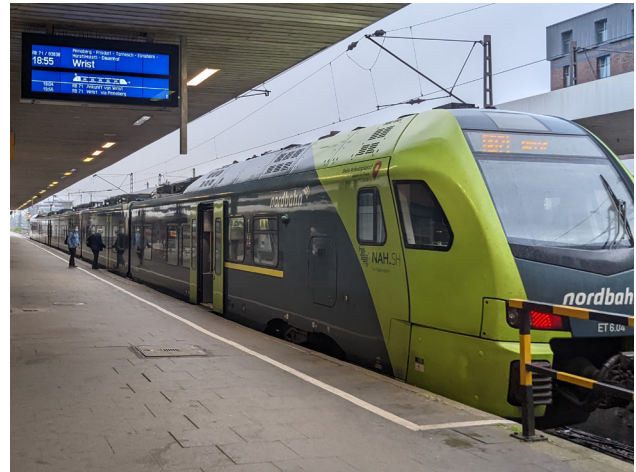
An electric multiple unit (EMU) train, pictured above in Germany, more closely resembles a subway train than the MBTA's current commuter rail fleet with large locomotives. Credit: Garth Frantzen for TransitMatters
